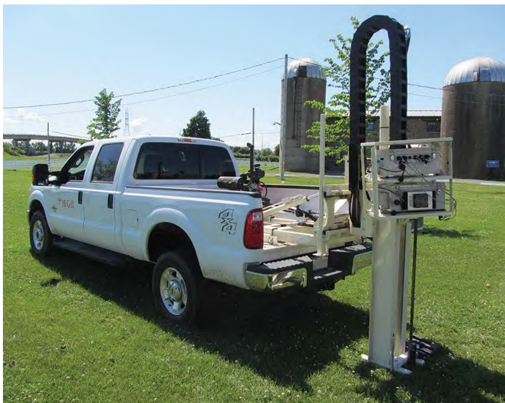
A probe equipped with insertion load sensors and two spectrometers, which cover visible and near infrared parts of the spectrum as well as electrical conductivity.
